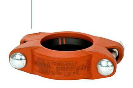
Figure 65HP extra heavy couplings are designed for high pressure service up to 1,000 psi; proof tested to 3 times maximum working pressure. As housings are tightened on the pipe, the tongue and groove design grips the pipe groove circumference providing a rigid joint connection. Bolt torques are cast into each coupling housing to simplify installation. Commonly used in oil field applications.
